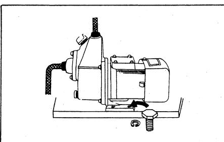
1 Being a stationary type, install the pump firmly at the required spot. The mounting feet are to be fastened by four bolts (8mm).
